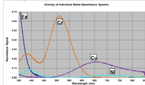
Fig. 3: Optical absorbance signals; Fe has a unique signal <~375nm. Cr has a unique signal at ~ 511nm. Cu has a fairly unique signal at ~ 850nm.
