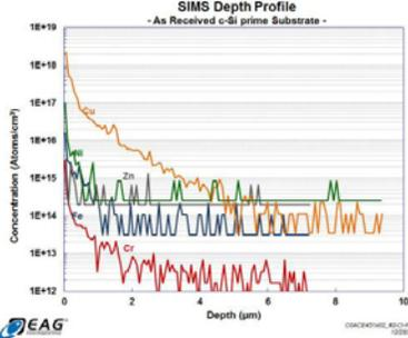
Fig. 1: SIMS depth profile of as-received c-Si prime substrate.
