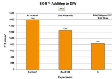
Fig. 2: 300ppm addition of SX-E to DIW rinse reduces surface Cu by 50% versus as-received wafers.
