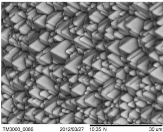
Figure 2. SEM of c-Si textured with additive A.
