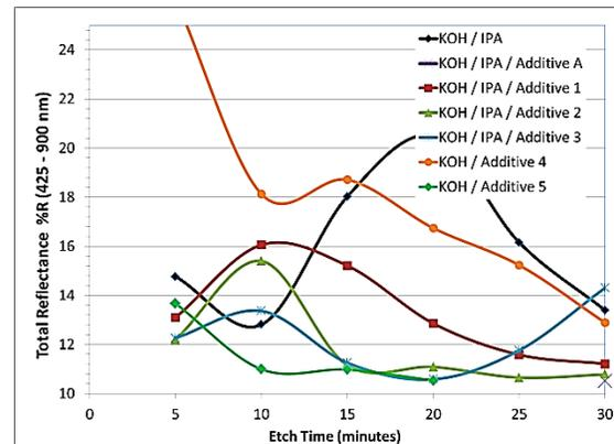
Figure 3. Reflectivity vs. etch time for different etch chemistries.
