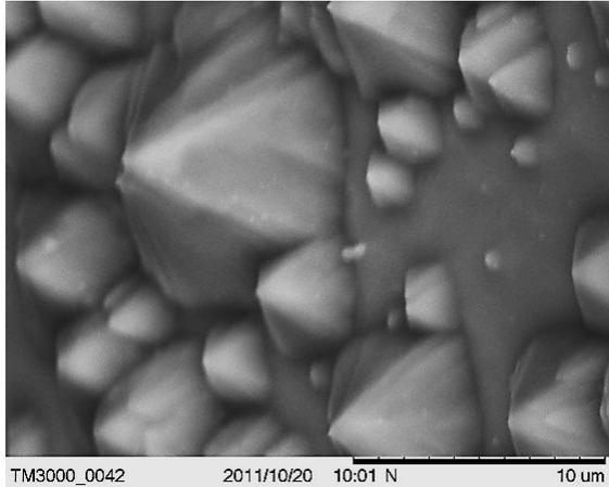
**Figure 5. Inhomogeneous etch by biodegradable texturing additive 4.**
