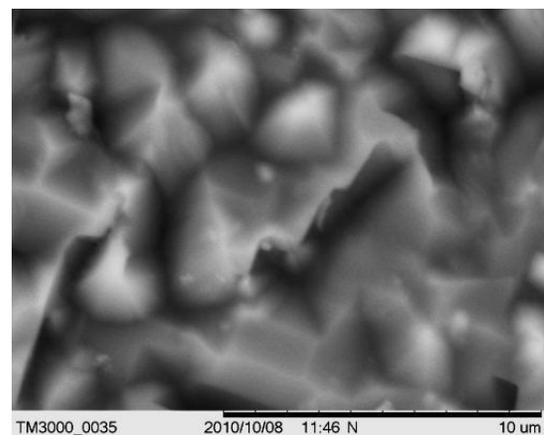
Figure 4. Loss of anisotropy by the use of biodegradable texturing additive 3.
