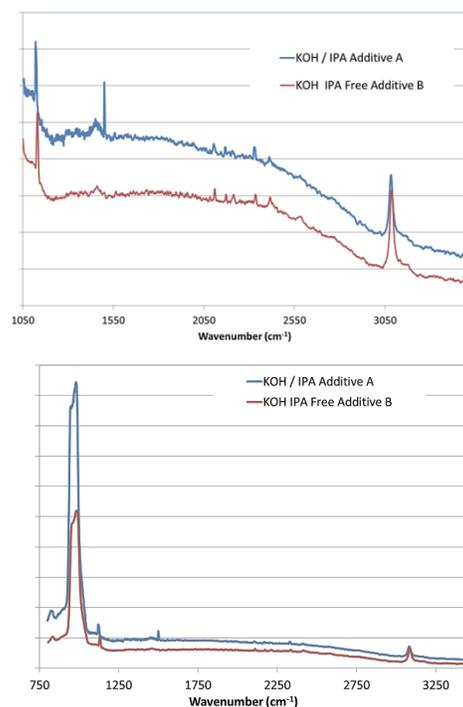
**Figures 1a and 1b. Raman Survey Spectra of texturing additive A residue on textured wafer prior to emitter diffusion.**
