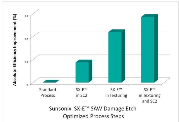
Figure 2: Cumulative improvements of SX-E™ as measured as the gain in absolute cell efficiency.
