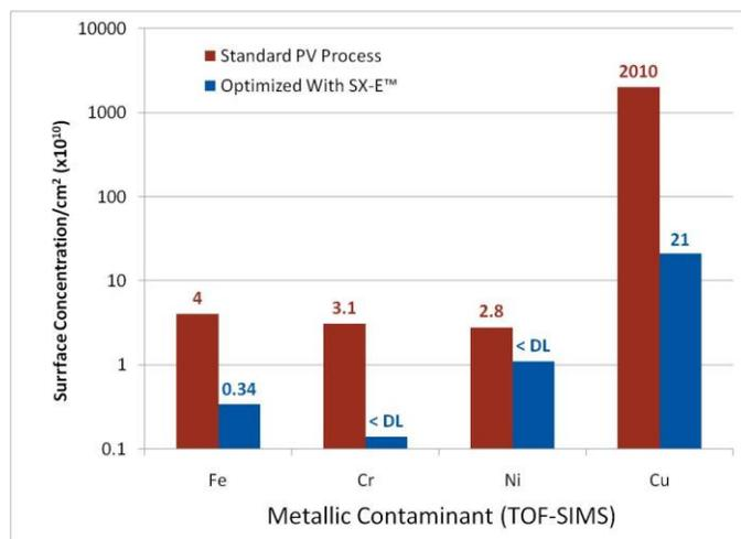
Figure 1: Surface metallic concentration for a standard PV saw damage etch (texturing) process sequence with and without SX-E™ optimized solution.
